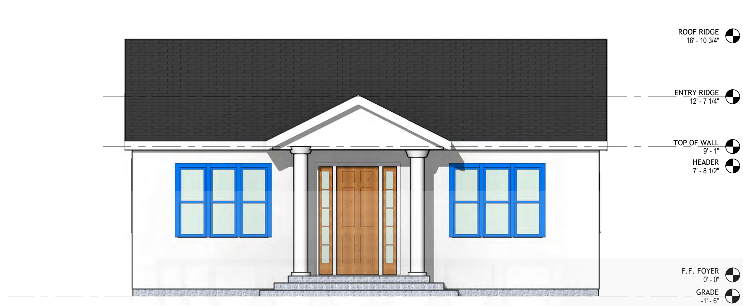
1 EX. FRONT ELEVATION 1/4" = 1'-0"
