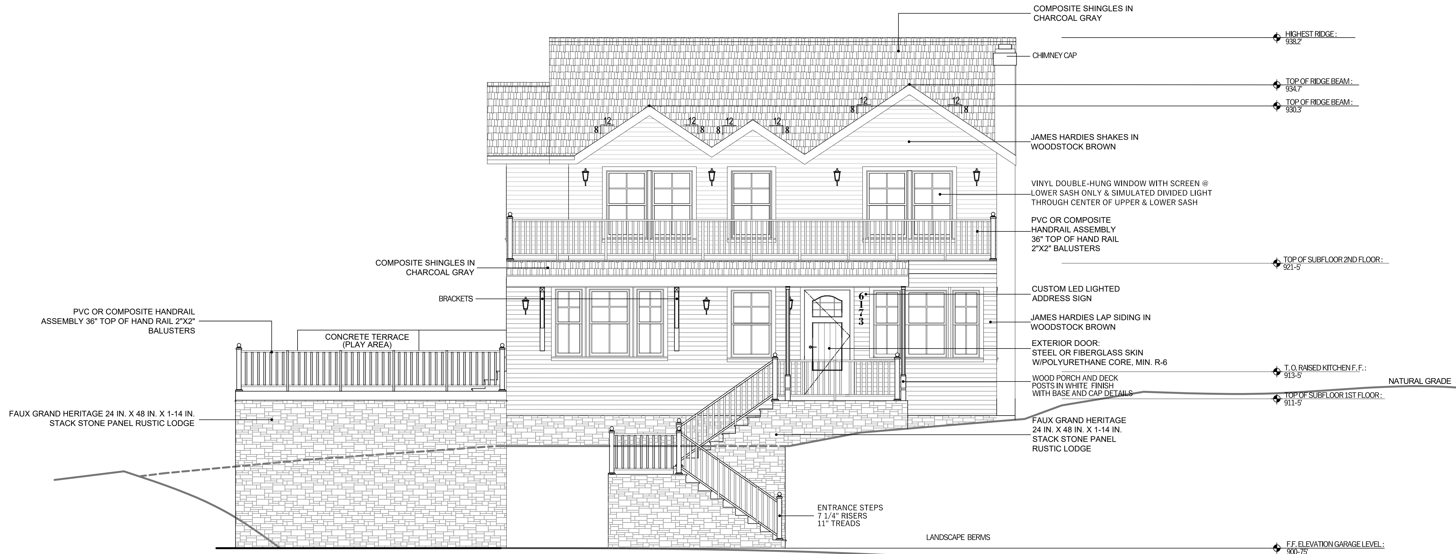
5 PROPOSED EAST (FRONT) ELEVATION Scale: 1/4" = 1' - 00"
