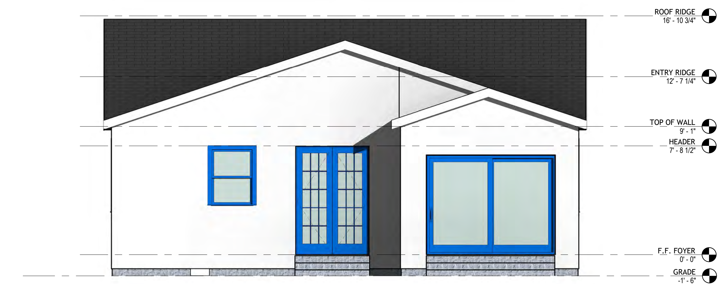
2 PR. REAR ELEVATION 1/4" = 1'-0"
