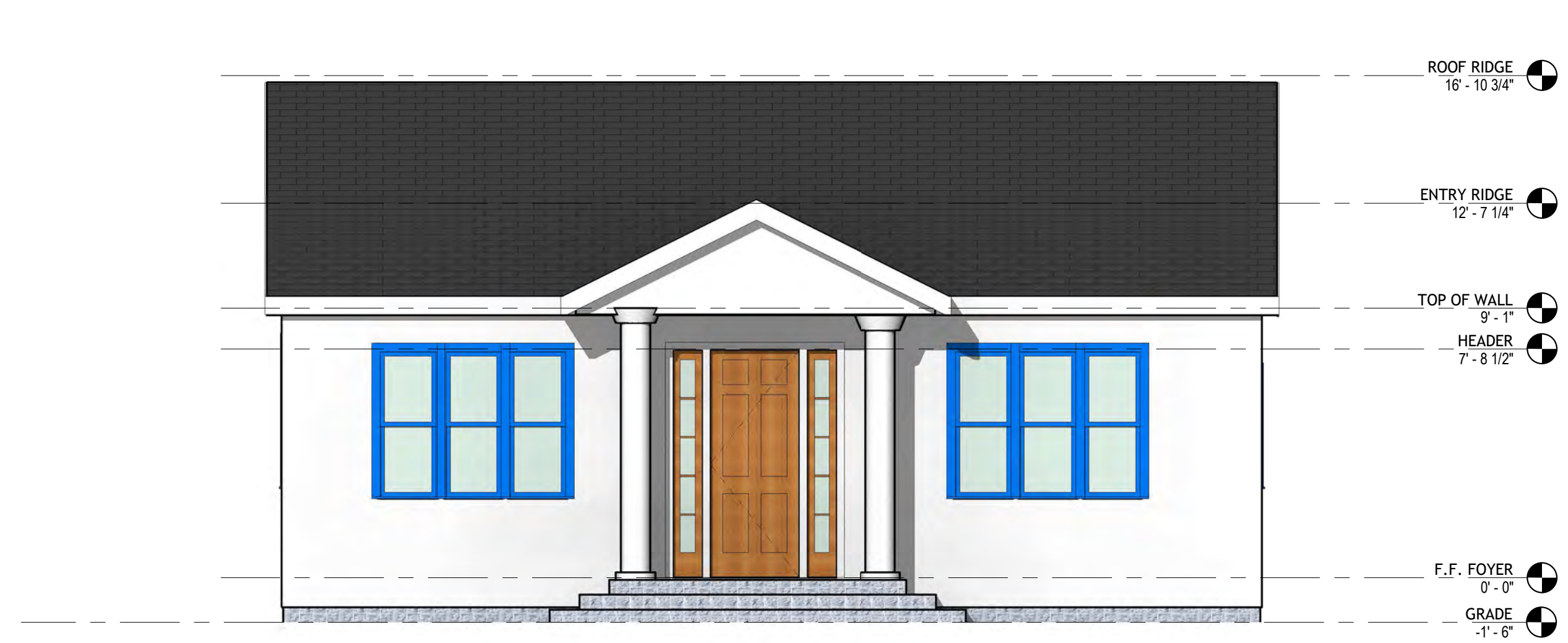
1 EX. FRONT ELEVATION 1/4" = 1'-0"
