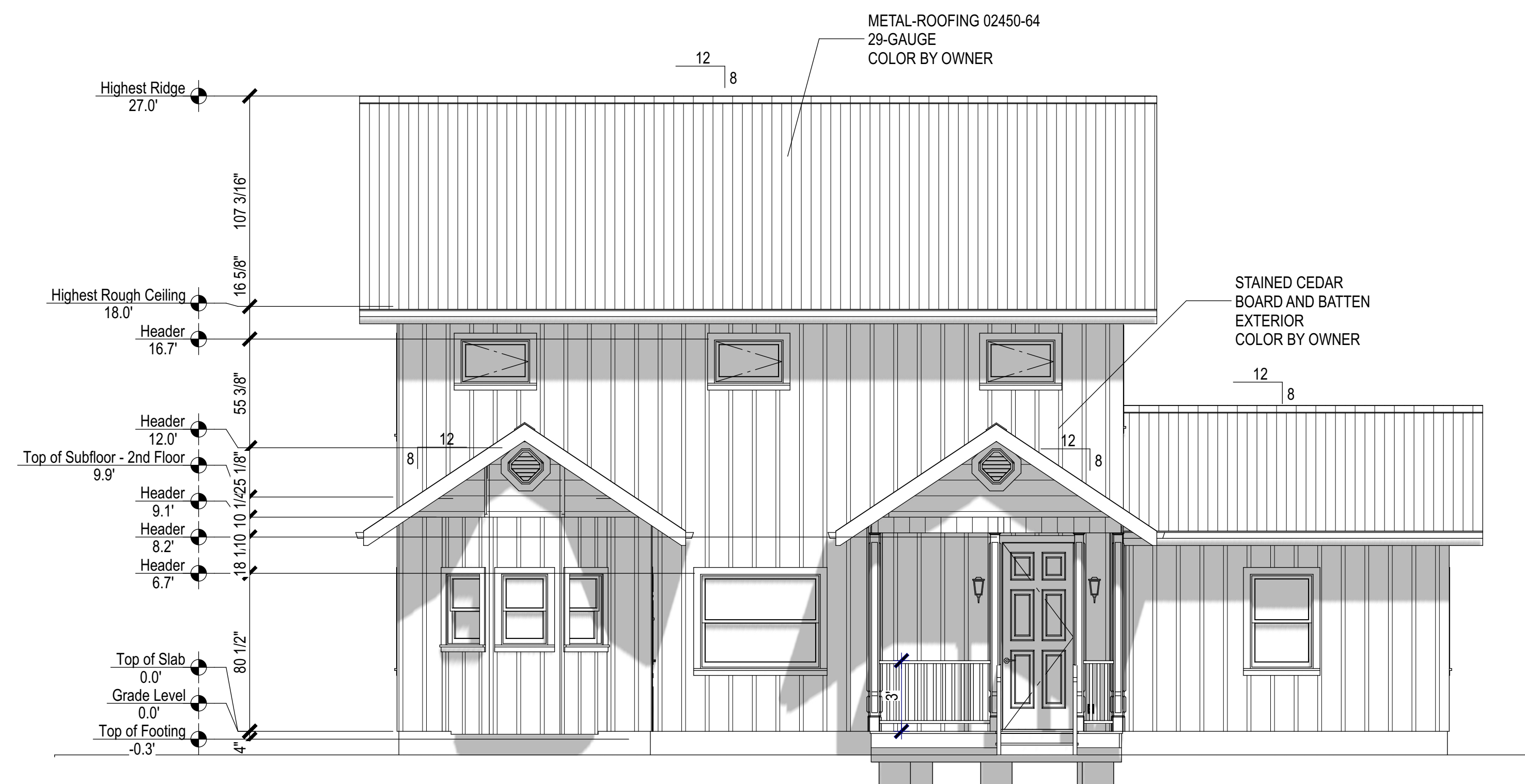
PROPOSED WEST ELEVATION SCALE: 1/4"=1'-00"
